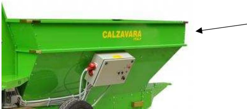
\***WETTER UNIT - BAGNATORE** A solenoid controlled automatic system that moistens the soil, peat, etc. when the blades turn. It is very effective in removing all the dust that forms during the processes.
