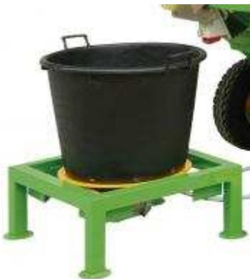
**\*WETTER UNIT** A solenoid controlled automatic system that moistens the soil, peat, etc. when the blades turn. It is very effective in removing all the dust that forms during the processes.
