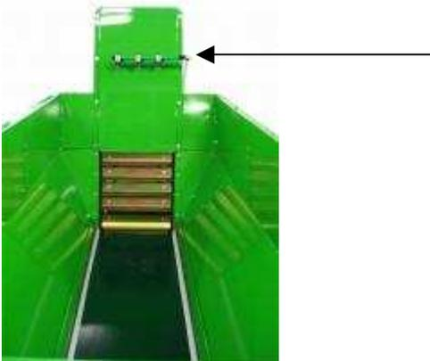
**\*SOIL LOADING BLADE MICRONS - MICRON CICLO PALE** A system for the operator to work the machine by just moving the vase against the micron. It has the same function as the pedals, but is in a practical position on the potting bench.
