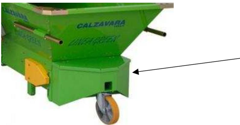
**\* VASE SUPPLY RACK – MAGAZZINO APP.TO VASI** An automatic system that deposits the vases directly on the machine distributor. It makes the operator's work smoother, as he does not have to constantly load the vases onto the machine but just onto the rack.
