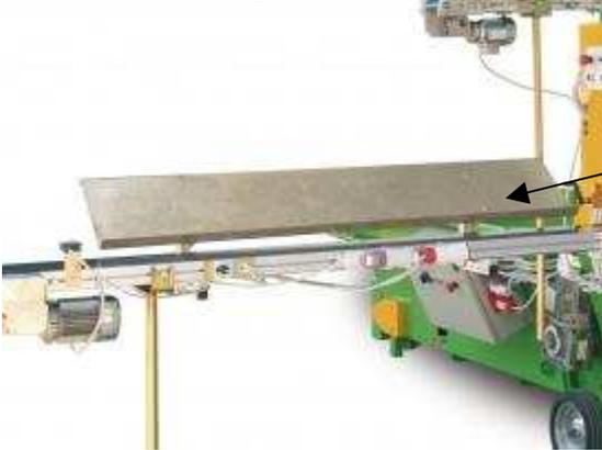
\* **SIDE FLAPS - SOVRASPONDE** Practical and strong to increase the machine loading capacity. (More or less 2,3 M3)
